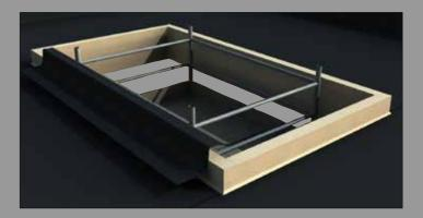
A timber kerb of 150mm high x 70mm wide (not supplied) must be fitted around the opening in the flat roof – the weatherproofing membrane laps onto the top face of the kerb.
